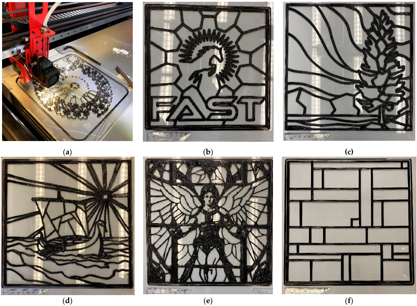
Figure 6. 3D printed stained glass sample designs with black PC filaments on clear PC sheets substrates of (a) Notre Dame rose window (SG01) during the 3D printing process and post-printing of: (b) FAST logo (SG02); (c) Northern Lights (SG03); (d) Viking Ship (SG04); (e) Angel (SG05); and (f) Geometric calibration pattern (SG06).
