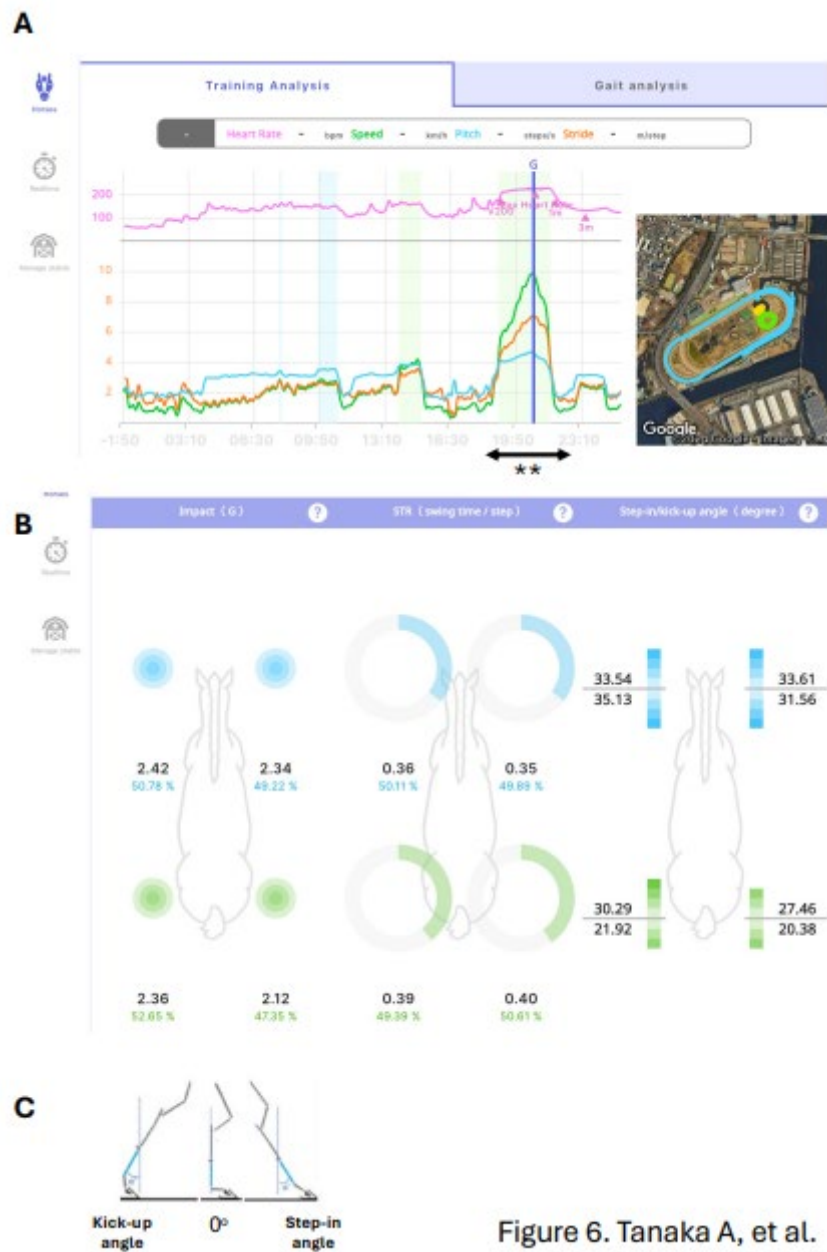
Figure 6. Training analysis screen displayed on the terminal (A). On the left is a line graph recording heart rate, speed, pitch, and stride during training, and on the right is a GPS showing the location of the run. Gait analysis screen displayed on the terminal (B). For each of the four limbs, the impact at ground contact, STR, and step-in/kick-up angle are displayed. (C) shows the principle of step-in/kick-up angle measurement.
