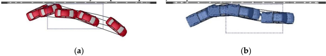
Figure 15. Vehicle trajectories impacting the TMBR at MASH TL-2 conditions: (a) 1100C; (b) 2270P.
