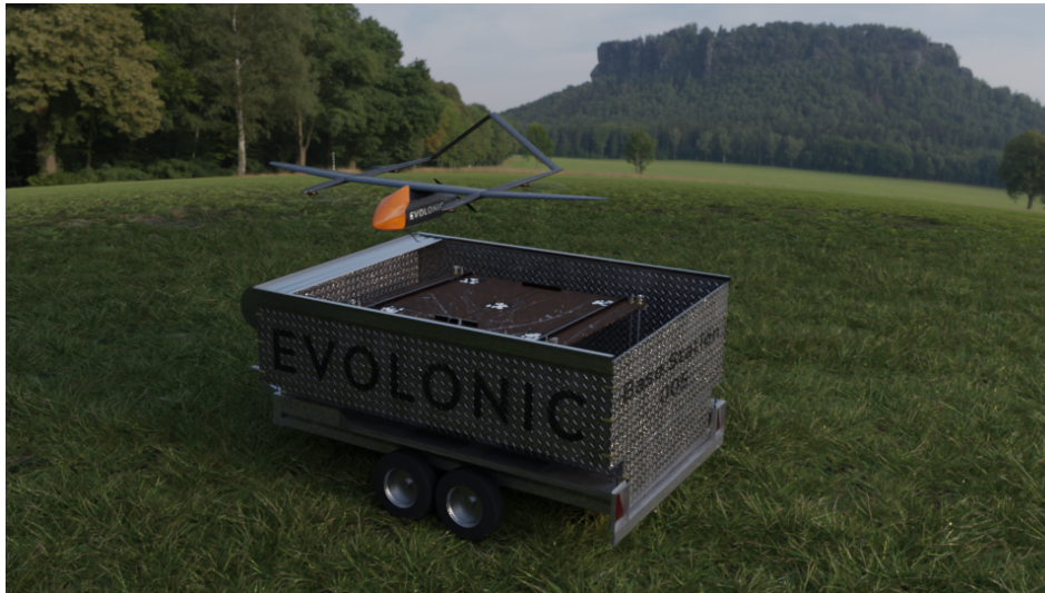
Figure 1. Rendering of the eVTOL drone that is used for this project with the base station
