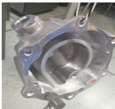
Figure 7. Impact Hammer Modal Testing Experiment.
