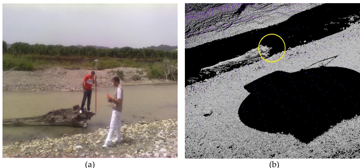
Figure 8. (a) GCP on a log in the Corace riverbed; (b) The same GCP in the point cloud. The purple dots on the shore are those acquired via ALS, as are the dots visible in the shadow area under the vehicle hosting the TLS.
