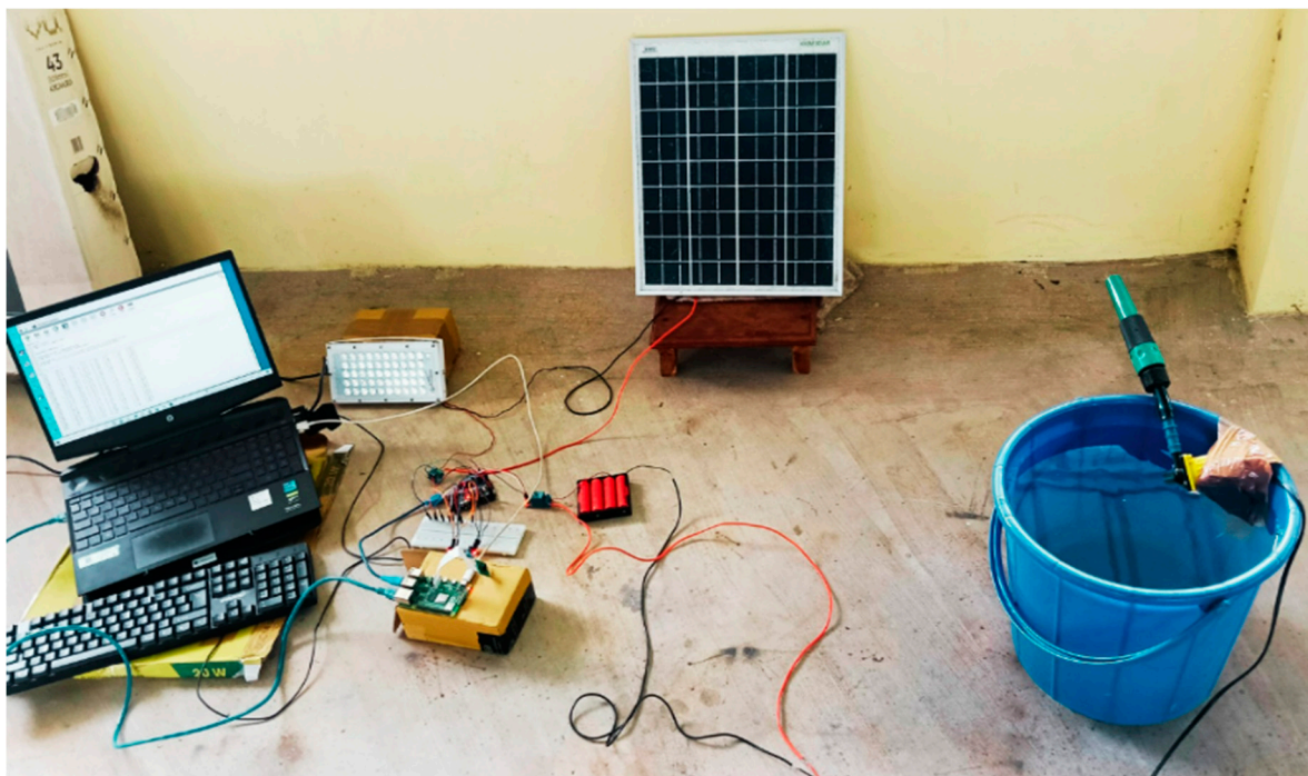
Figure 23. Complete experimental setup with solar panel and cleaning system.
