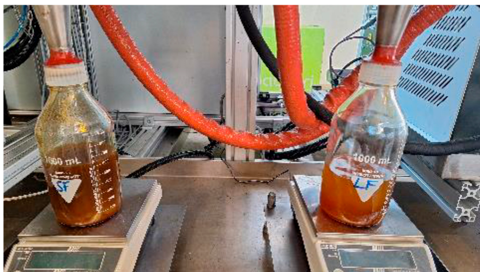
Figure 7. Pyrolysis oil fractions obtained during the experiment: left, heavy oil (HF); right, light oil (LF).
