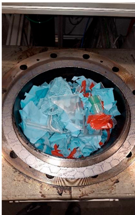
Figure 2. Shredded plastic waste from the TUR tray placed in the experimental reactor.
