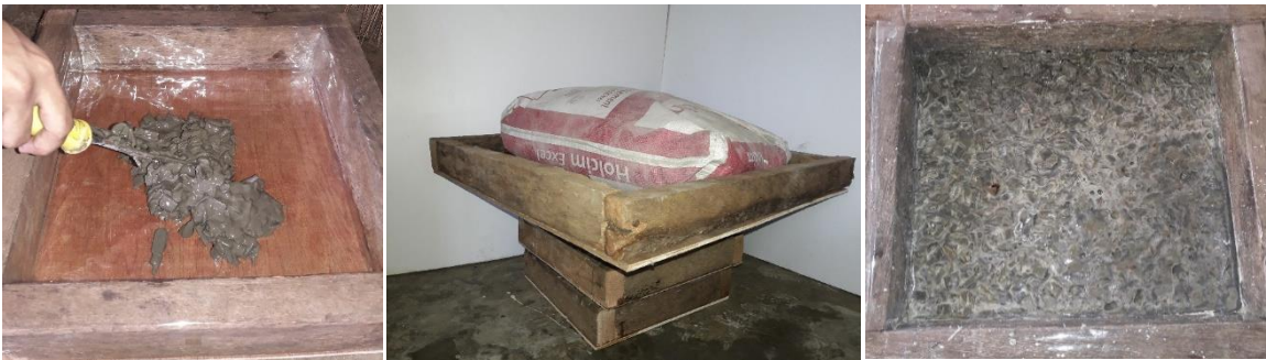
Figure 1. (left) Spreading the mixture in a wooden mould; (middle) Placing a weight on top of the samples and leaving it there for 24 hours; (right) Cured COPAP samples ready for testing
