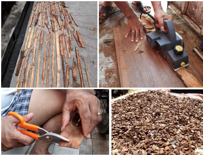
Figure 2. (Upper left) Sundried barks of Cocos nucifera ; (upper right) Extraction of phellem from the sundried barks using a wood planer; (bottom left) Cutting of extracted phellem into smaller uniform sizes; (bottom right) Trimmed phellem pieces sun-dried once more to remove any remaining moisture.
