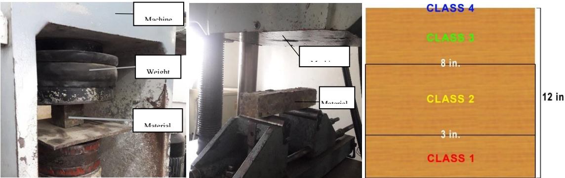
Figure 4. (left) 2" x 2" COPAP board specimen loaded on a self-aligning loading block ready for a compressive strength test; (middle) 2" x 2" x 12" COPAP board specimen on a loading block for a flexural strength test; (right) Flame Spread Classification Guide showing the lengths that determine the flame spread rating of a material.
