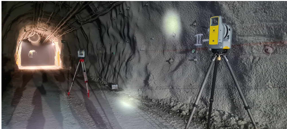
Figure 4. TLS measurement of underground mining tunnel.
