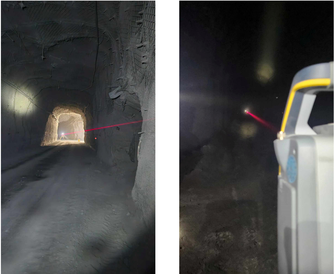
Figure 3. Check survey during traverse network measurement.
