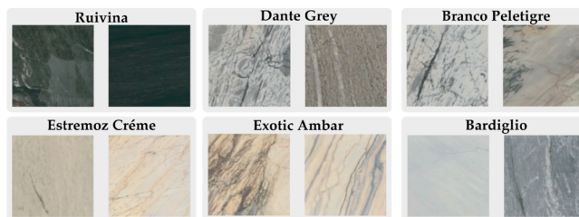
Figure 2. Examples of intra-class visual variability are present in the dataset. Images within the same commercial variety exhibit substantial differences in veining density, base color, and textural organization.
