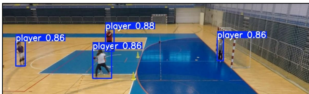
Figure 3. Example of player detections in a broadcast handball frame using YOLOv8.
