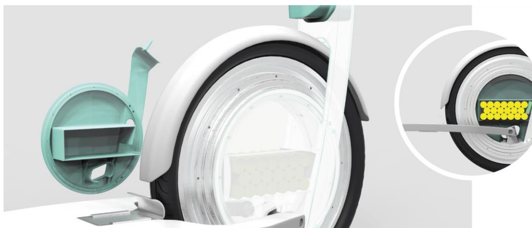
Figure 10. Overview of the fixed battery case configuration.
