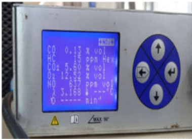
Figure 4. Flue gas analyser- A DIGAS 444 N.
