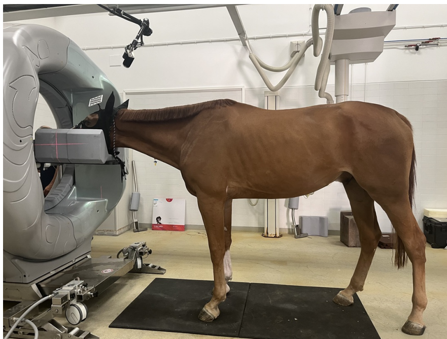
Figure 1. Sedated horse positioned for standing equine CBCT of the head region. A ChArUco board is rigidly attached to the horse's head and observed by the RGB camera for external pose tracking during acquisition.
