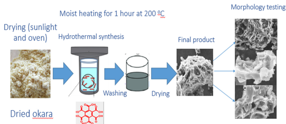
Figure 3. HTC method and procedure to prepare hydrochar.
