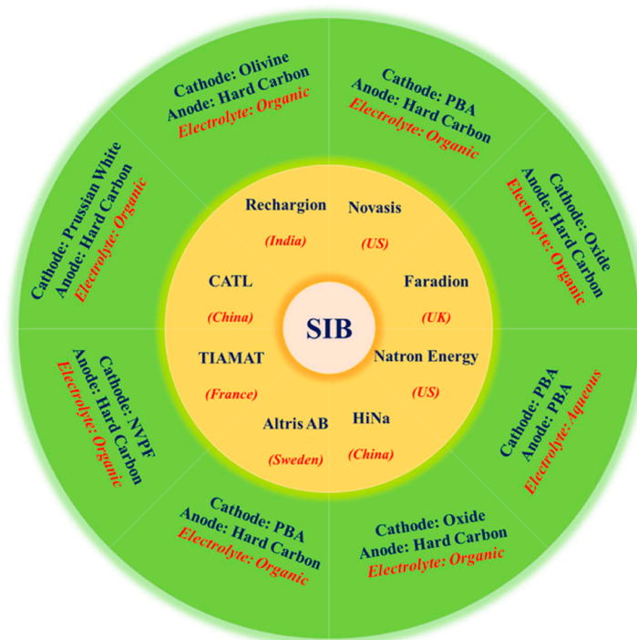
Figure 4. Schematic overview of key industrial sodium-ion battery (SIB) developers and the electrode/electrolyte combinations commonly reported for their commercial platforms (layered oxides, Prussian blue analogues, and polyanionic cathodes; typically paired with hard carbon anodes; organic or aqueous electrolytes depending on the system). (Adapted with permission from ref. [63], Oxford Academic, 2023).
