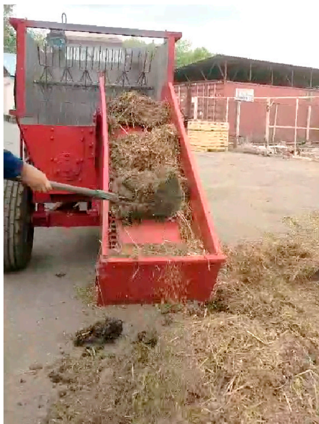
Figure 6. Fragment of loading feed components into the hopper of the feed mixer-distributor using the conveyor.
