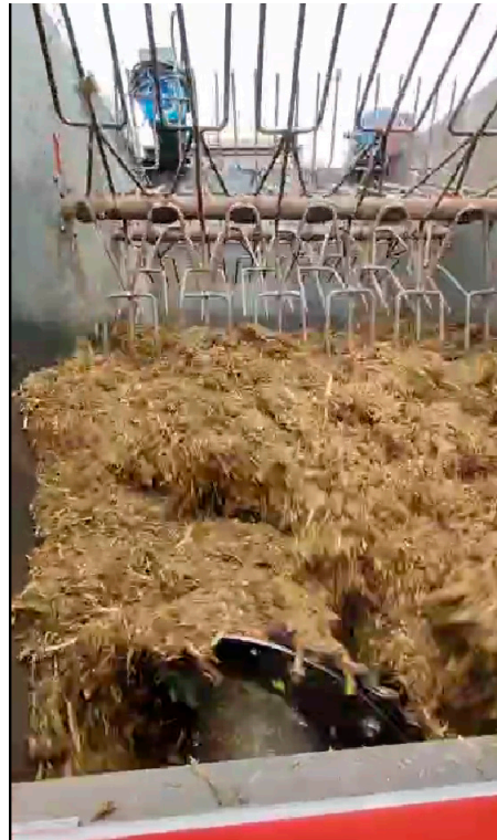
Figure 10. Position of the leveling-mixing finger shaft at the initial stage of feed mass discharge.
