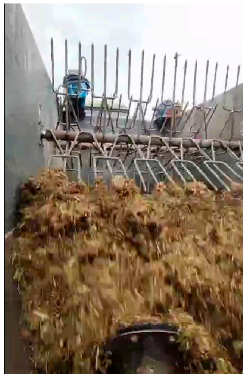
Figure 11. Position of the fingers of the leveling-mixing shaft at the final stage of feed mass discharge.
