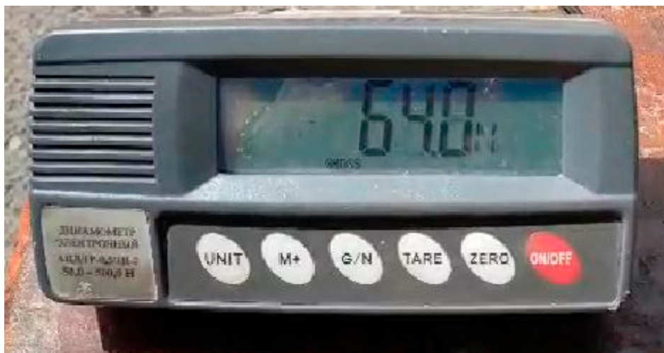
Figure 13. Instantaneous values of the resistance torque during operation of the machine equipped with the leveling-mixing device.
