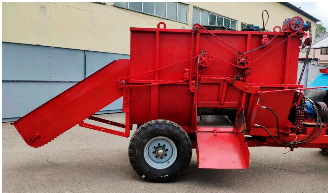
Figure 3. General view of the experimental prototype of the compact feed mixer-distributor. Factory tests of the feed mixer-distributor were carried out. It was established that all mechanisms operated under the specified operating conditions, and the machine was confirmed to be ready for field testing and experimental investigations.
