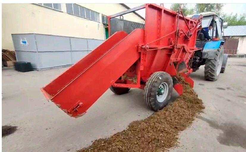
Figure 7. Fragment of the experimental technological process of unloading the feed mixture onto the feeding table.
