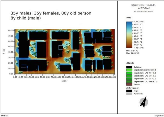
Figure 21. ENVI-met simulation of the area of study, UTCI 10 a.m., male 35y, female 35y, old person male 80y and child male 8y.
