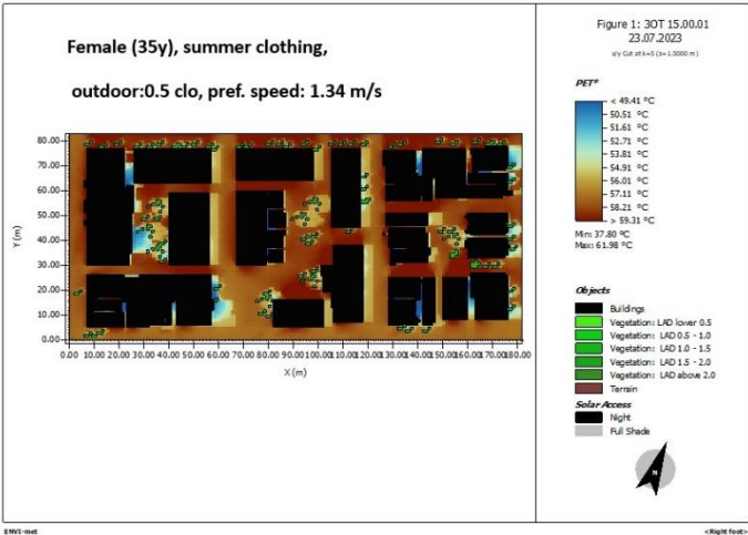
Figure 14. ENVI-met simulation of the area of study, PET 3 p.m., female 35y, summer clothing, 0.5 clo, pref.speed 1.34 m/s .
