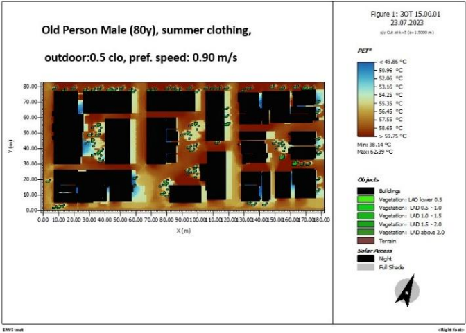
Figure 15. ENVI-met simulation of the area of study, PET 3 p.m., old person male 80y, summer clothing, 0.5 clo, pref.speed 0.90 m/s.
