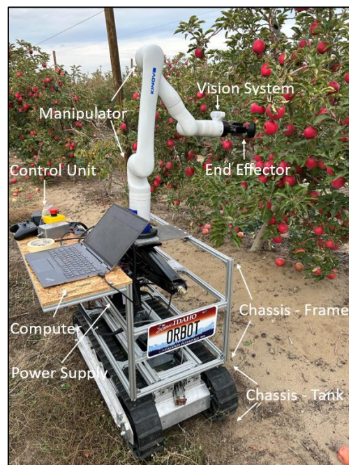
Figure 1. Orchard Robot (OrBot) and its subsystems.
