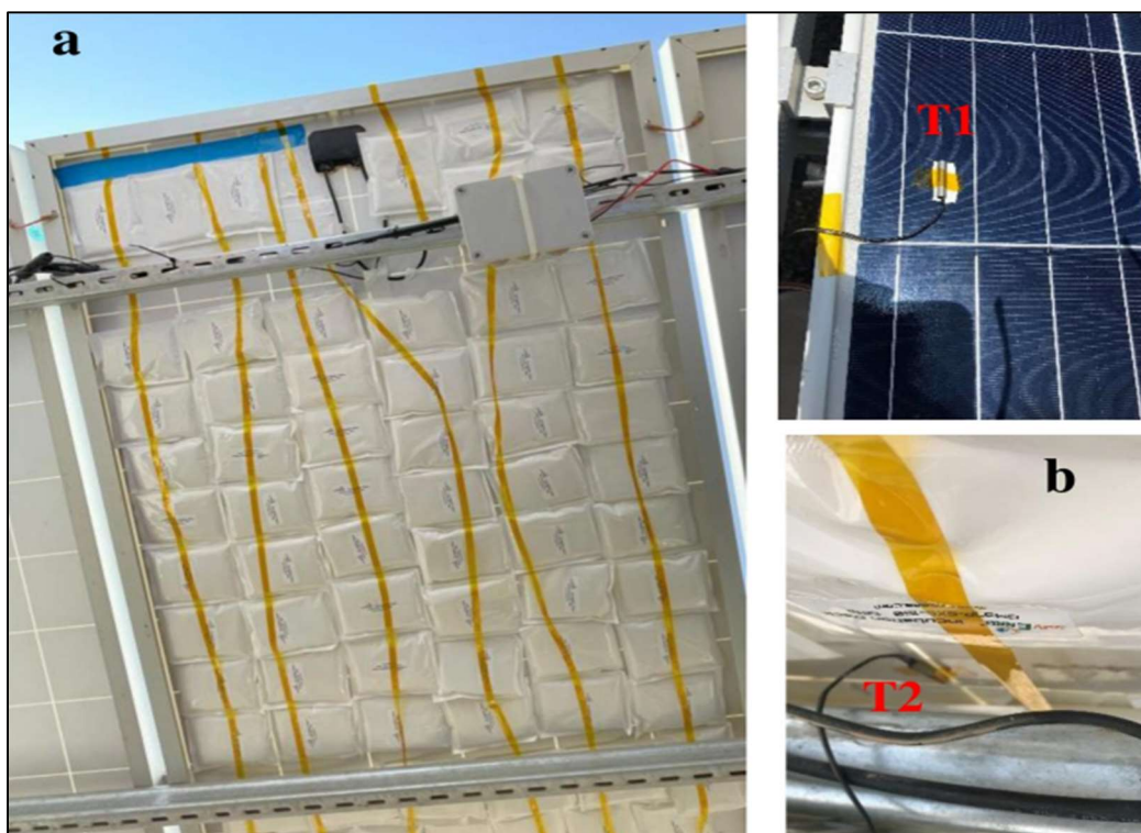
Figure 37. a) PCM packs filled with PCM-OM37P substance b) Positioning of the front and rear thermocouples.
