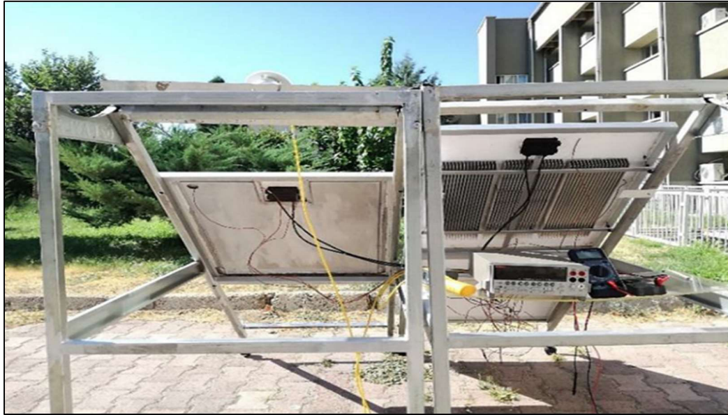
Figure 40. Rear view of photovoltaic systems: PV + PCM on the left, PV + fin3 on the top right, and reference PV on the bottom right. The systems are located at 36° and 42° North latitudes.
