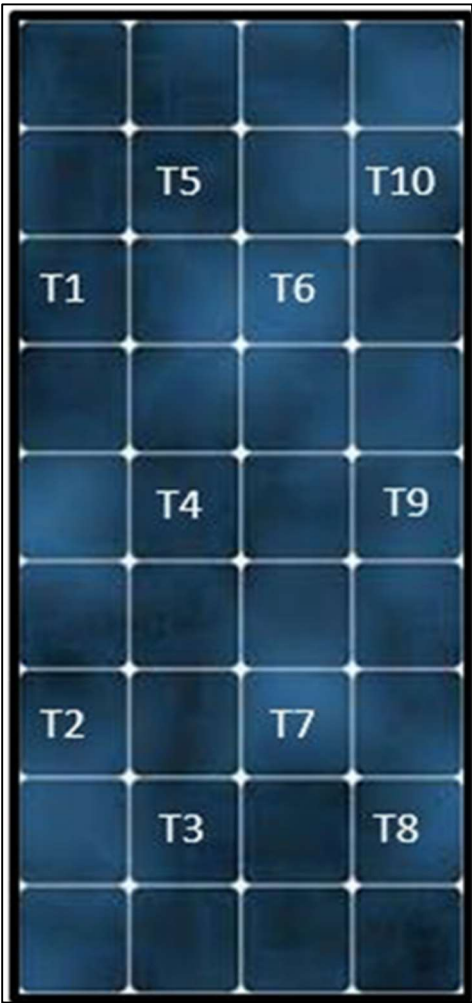
Figure 41. Displays the arrangement of the thermocouples on the photovoltaic panels.
