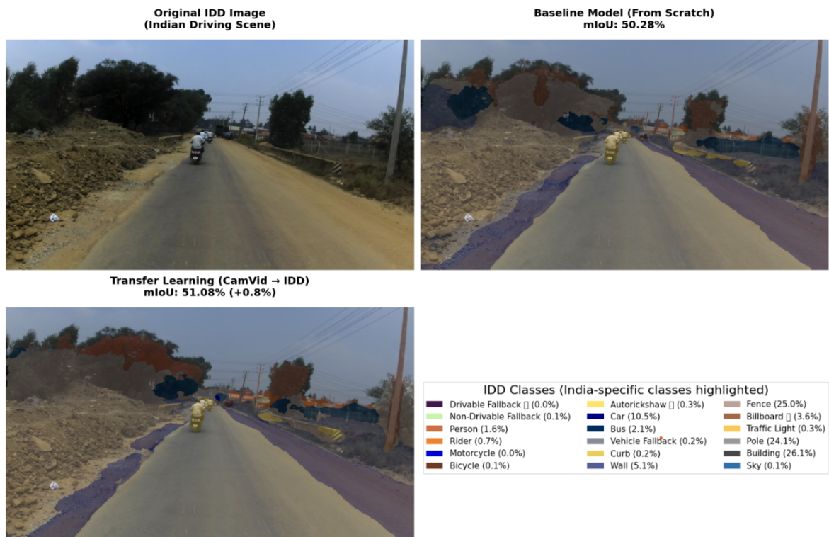
Figure 13. Prediction overlays on IDD dataset: Top—baseline prediction; Bottom—transfer learning from CamVid. Improved detection of road area, vegetation, and person classes.
