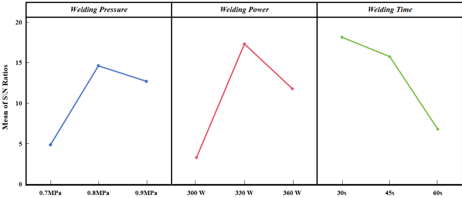
Figure 3. Main effect diagram of single lap shear strength of CF/EP welded joints.
