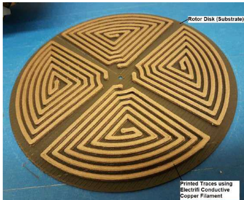
Figure 16. Copper impregnated PLA coils extruded onto a ProtoPasta™ pancake rotor.
