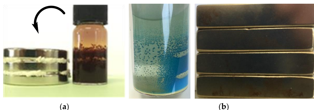
Figure 1. (a) Crystallisation pattern of [Ni(dppf)Cl_2] , 1 , inside a stack of three ring magnets (b) A vial containing a crystallising solution of [(C_6H_4-CH_2P^tBu_2-2-C_6H_4-CH_2P(H)^tBu_2)_2NiCl_3] placed adjacent to a stack of 4 magnets. Smaller crystals are observed next to the magnet and distinct areas of little or no crystallisation is apparent.
