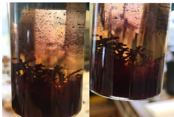
Figure 6. Crystallisation of [\text{Ni } P,P\text{-}(\eta^2\text{-triphos})\text{Cl}_2] showing the crystals reaching into solution following field line patterns. These crystals form suspended fragile grids which collapse on agitation.
