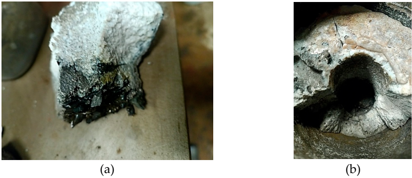
Figure 9. Image of the crucible contents after the reaction in section: a) side view; b) top view.
