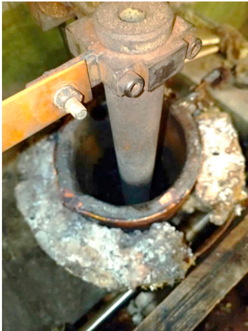
Figure 6. Illustration of the installation for electroslag reduction of cadmium from CdO with carbon.
