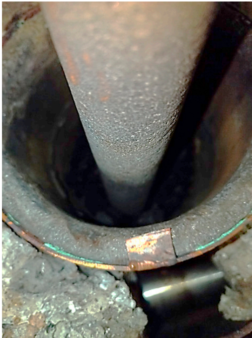
Figure 4. Image of a crucible filled with carbon before adding liquid KCl-NaCl (KN) flux and CdO.
