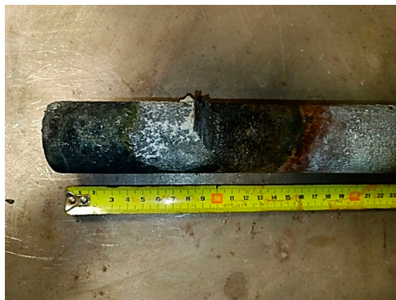
Figure 8. Image of a graphite electrode removed from the melt after melting, showing three zones.
