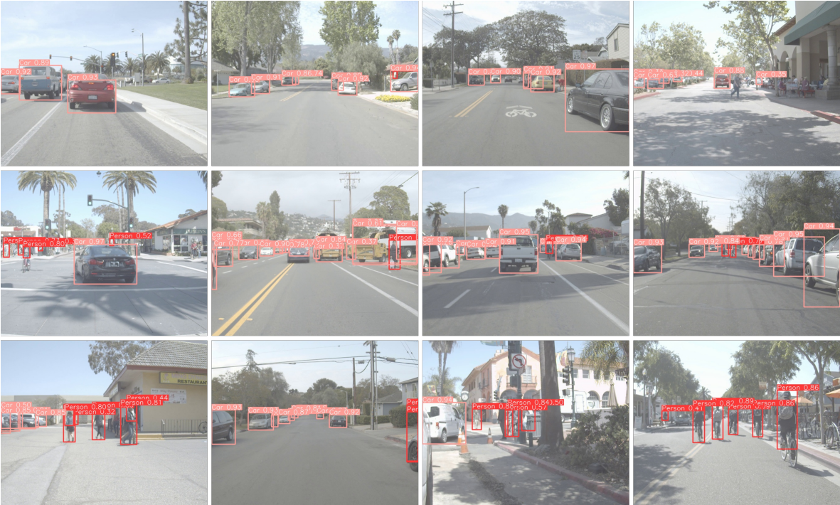
Figure 12. Detection results of CMAFNet on RGB images from the FLIR-Aligned dataset. The model demonstrates accurate detection of Person, Car, and Bicycle categories across various urban driving scenarios with different lighting conditions and traffic densities.
