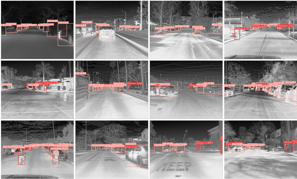
Figure 13. Detection results of CMAFNet on IR images from the FLIR-Aligned dataset. The thermal infrared images clearly reveal pedestrians and vehicles through their heat signatures, enabling reliable detection in nighttime and low-visibility conditions.
