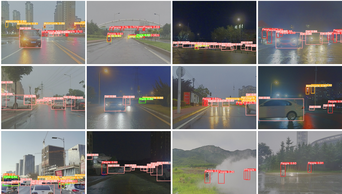
Figure 10. Detection results of CMAFNet on RGB images from the M3FD dataset. The results demonstrate robust detection across diverse scenarios including daytime, nighttime, rainy, and foggy conditions. CMAFNet accurately detects multiple object categories including People, Car, Motorcycle, Bus, and Truck with high confidence scores.
