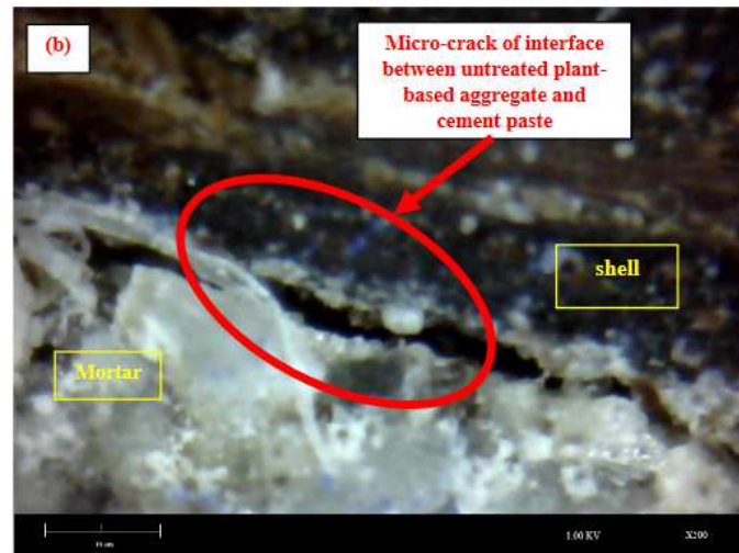
Fig. 9. (a) Pre-treated grout soaking and (b) untreated interfacial bonding between the cement paste and shell aggregate
