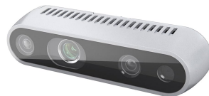
Figure 9. Structured light depth-sensing camera for object detection and spatial awareness
