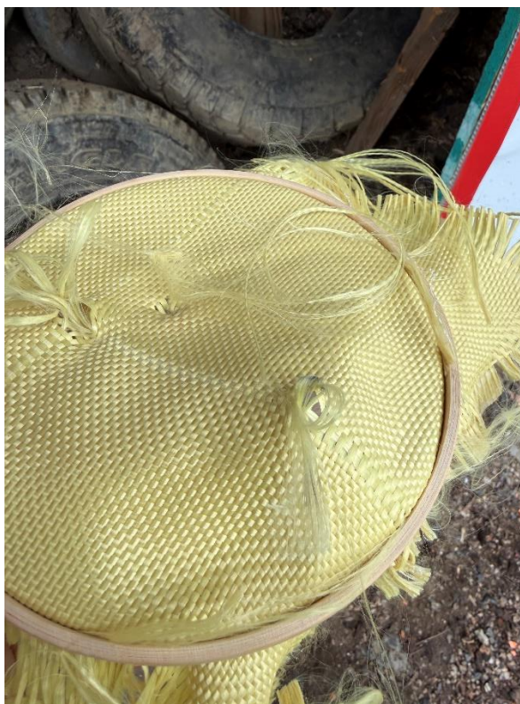
Figure 12. Visual damage to the Kevlar sail after ballistic testing.
