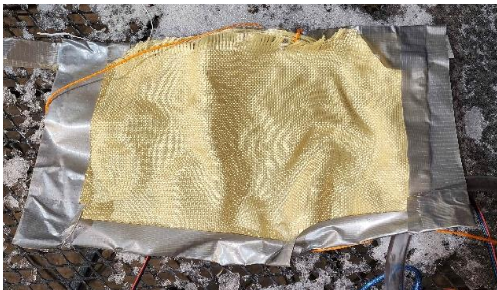
Figure 7. Kevlar sail for ballistic interception.
