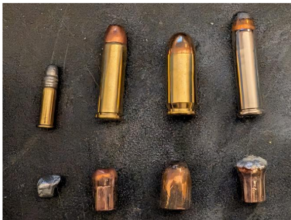
Figure 11. Comparison of standard rounds (top) with recovered bullets (bottom). Left to right: .22 Long Rifle (LR), .38 Special, .45 Automatic Colt Pistol (ACP), and .357 Magnum.
