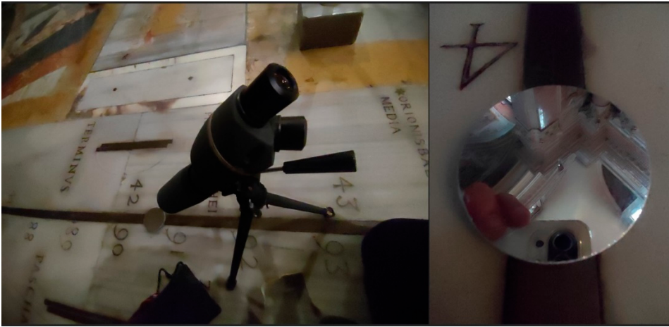
Figure 11. The telescope and the flat mirror reflecting the pinhole, on the meridian line.
