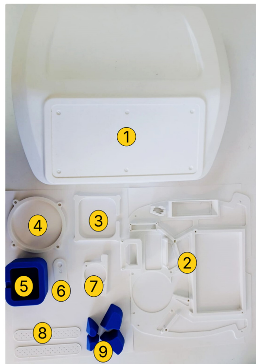
Figure 5. Housing and accessories. E1) Housing. E2) Internal base housing. E3) Top holder. E4) Fan bracket. E5) Protective cover. E6) VNA port cover. E7) Back fan trim. E8) Vent cover. E9) Legs.
