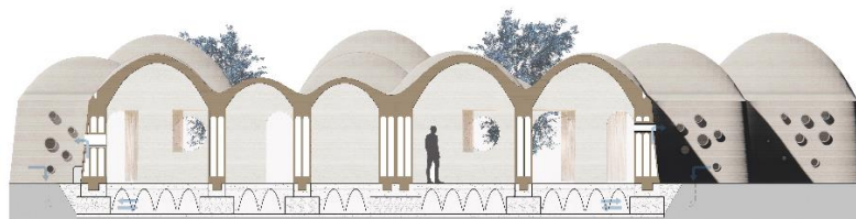
Figure 22. Section B-B' (Figure 17) with air recirculation.
