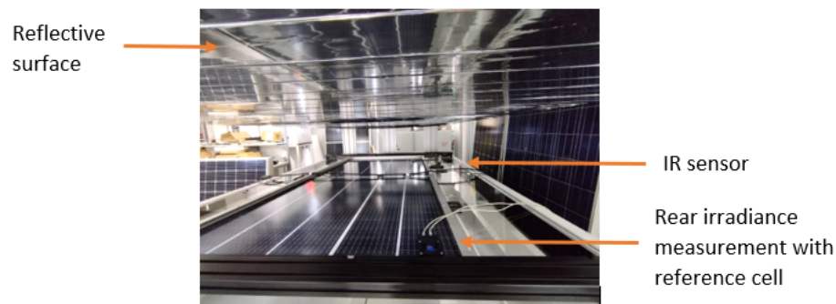
Figure 5. Solar simulator setup for double-sided measurement.
