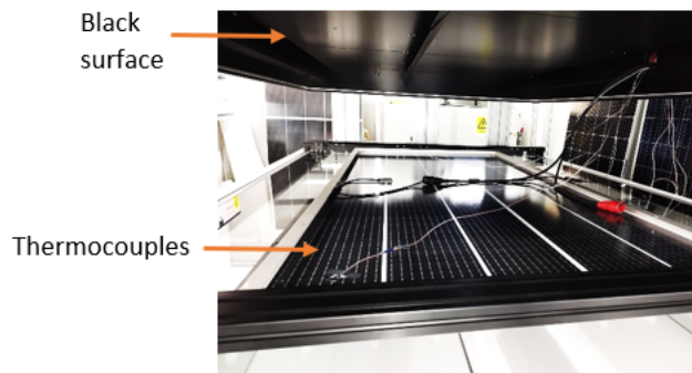
Figure 4. Solar simulator setup for single-sided measurement.
