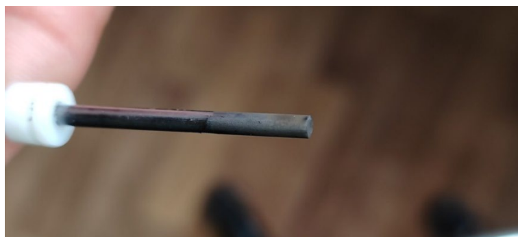
Figure 9. Image of the graphite electrode after multiple operation of the thruster.
