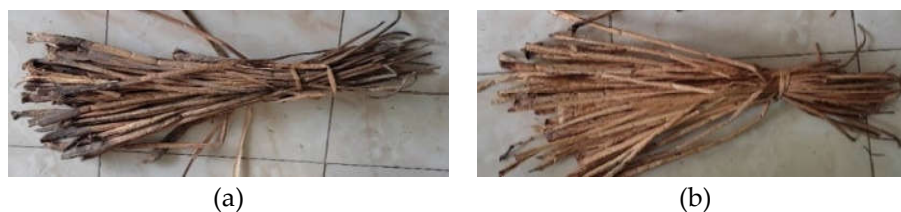
Figure 11. Results of Dried Water Hyacinth, (a) Using Manual Method; (b) Using Dryer Machine.
