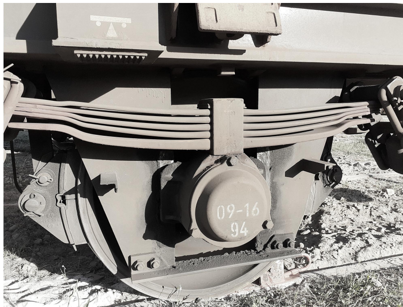
Figure 1. Parabolic leaf springs usually found in UIC two-axle freight wagons.
