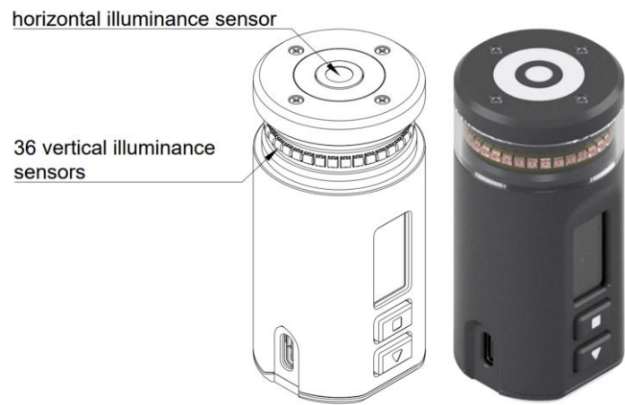
Figure 3. Proposed construction of multi-sensor cylindrical illuminance sensor, drawing and model render.
