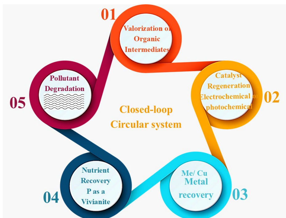
Figure 5. Closed-loop circular system for advanced oxidation and resource recovery.
