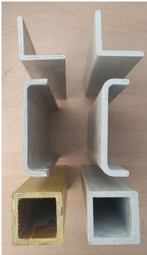
Figure 5. Kenaf/glass fibre reinforced pultruded hybrid profiles (left) and glass fibre reinforced pultruded profiles (right).
