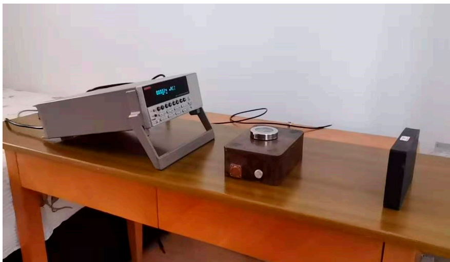
Keithley 6514 ( 10^{-16}A ) a copper shielding box a magnet (There is a compass on the top of the copper box, showing the direction of the magnetic field.) (2) The arrangement within the copper shielding box
