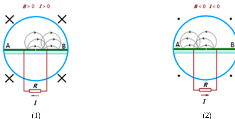
Figure 6. An electric potential demon. (1) When the direction of the magnetic field enters into the paper, the output current is positive. (2) When the direction of the magnetic field leaves out the paper, the output current is negative.
