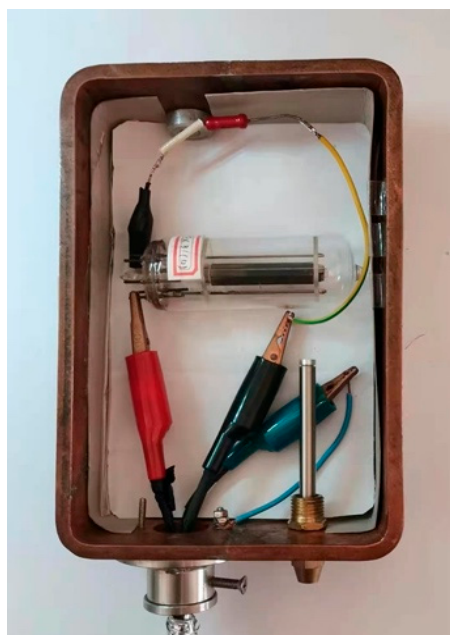
Keithley 6514 ( 10^{-16}A ) a copper shielding box a magnet (There is a compass on the top of the copper box, showing the direction of the magnetic field.) (2) The arrangement within the copper shielding box
