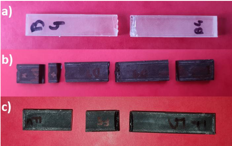
Figure 5. Fractured specimens after three-point flexural test: a) 0% rGO, b) 2% rGO, c) 0.25% rGO.
