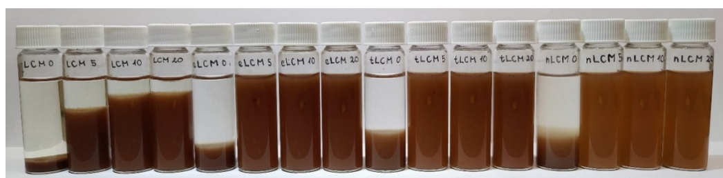
Figure 2. The stability of the non-sonicated (0 min) and sonicated (5, 10, 20 min) LCM, eLCM, tLCM and nLCM suspensions after 72 h from their preparation.
