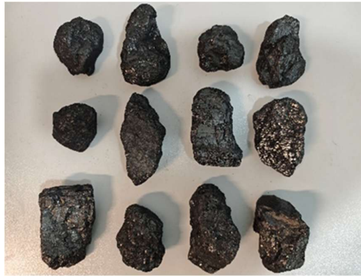
Figure 2. Sample Diagram Showing Partial Particle Size Ranging from 40 to 50 mm.
