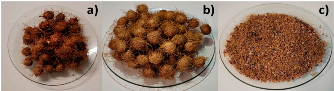
Figure 3. Açai seeds after physical pre-treatment. Legend: seeds + fibers (a); seeds + dry fibers (b); comminuted seeds (c).
