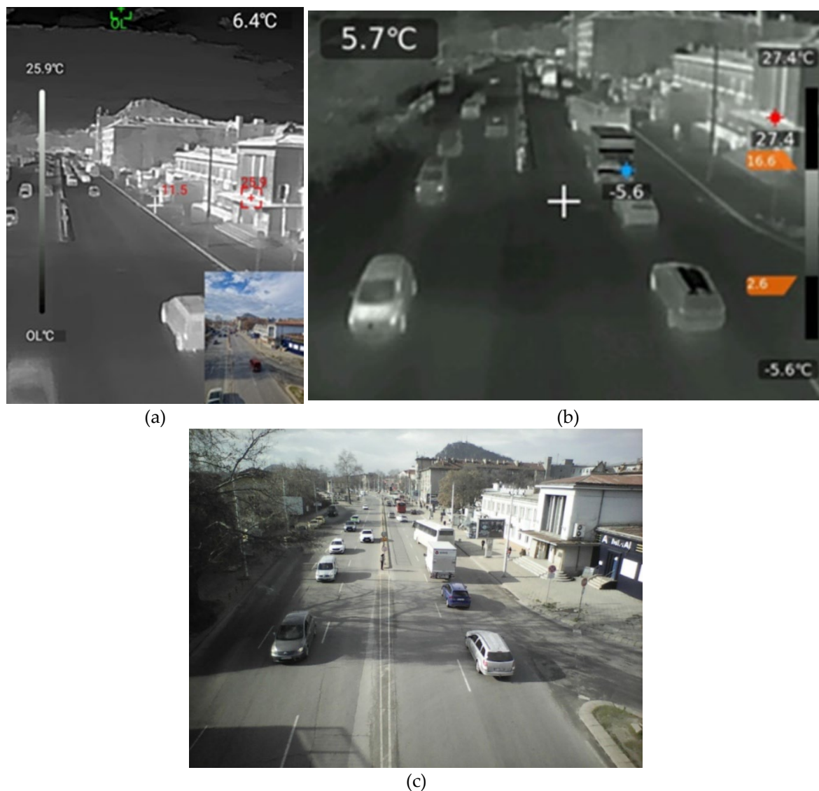
Figure 12. Example demonstrating practical observation range and scene coverage for UTi260M and synchronized dual-channel capture with UTi260T: (a) UTi260M with smartphone and application; (b) thermal frame used for temperature-contrast and detectability assessment; (c) simultaneous visible-light frame used to document illumination conditions and scene context (road geometry, traffic, and glare sources).
