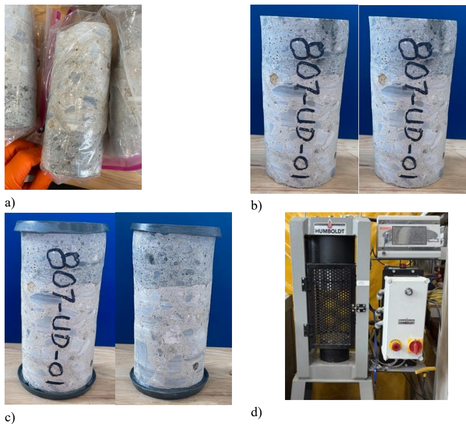
Figure 3. Bridge core samples a) bagged bridge core from DelDOT b) bridge cores before c) after capping d) Humboldt compression machine.
