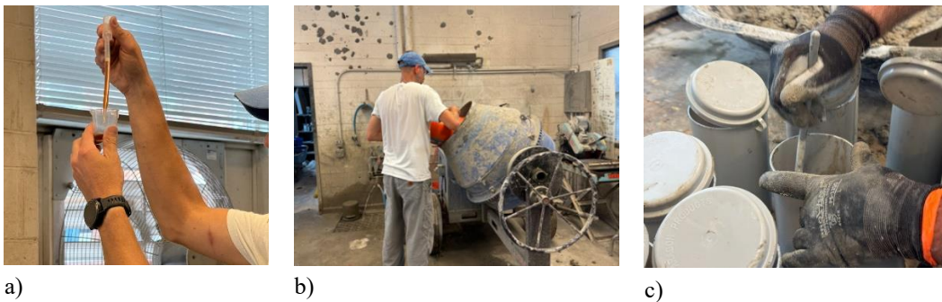
Figure 1. Sample preparation a) Measuring of the air entrainer admixture b) Concrete mixer c) Casting of Concrete Sample.
