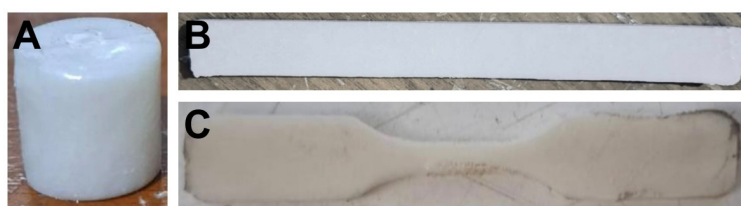
Figure 2. 3D-printed scaffolds. (A) Compression tests' specimen. (B) Bending tests' specimen. (C) Tensile tests' specimen.
