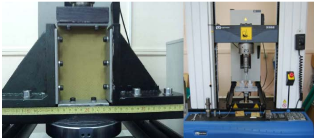
Figure 3. In-plane compression and anti-buckle Rig, Test frame.
