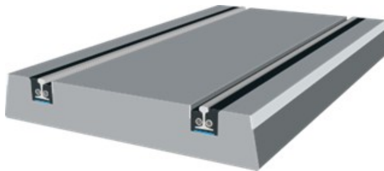
Figure 2. Track with continuously fastened rails [25].
